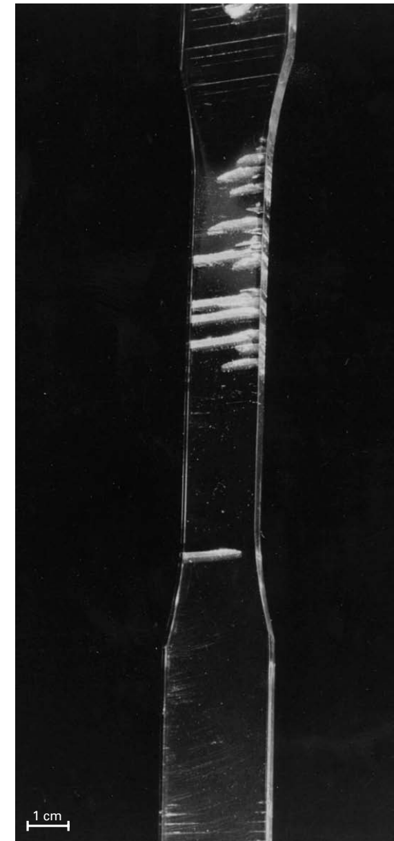
Fig. 8.43 A series of crazes produced in a tensile specimen of polycarbonate. (Used with permission from R. P. Kambour, Polymer , 4 (1963) 143.)
