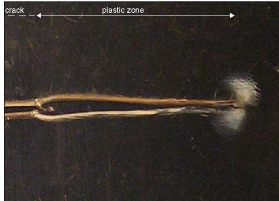
Fig. 11.6 Craze region at tip of plastic yield zone ahead of an edge crack in thin sheet of polycarbonate. (The white region along the crack and the long plastic zone is reflected light due to the oblique angle of exposure (out of the plane of the page))
