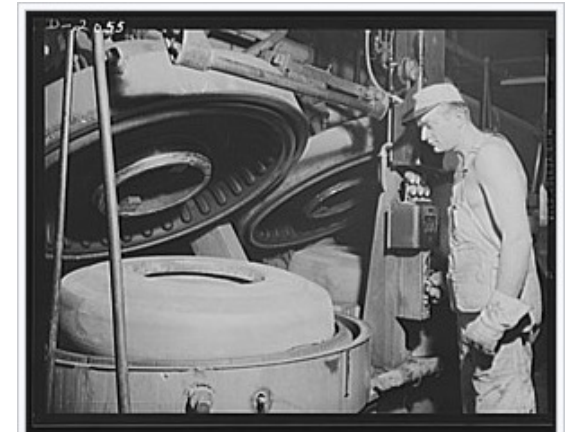
Worker placing tire in a mold before vulcanization.
