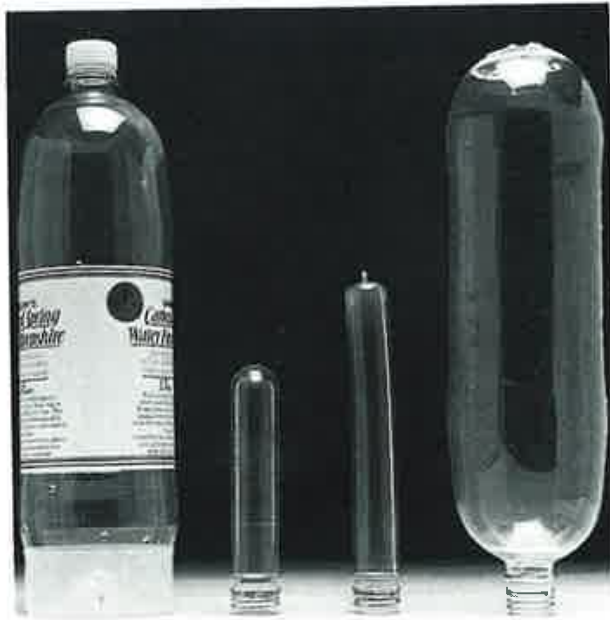
Figure 5.46 A complete 1.5-litre poly(ethylene terephthalate) bottle, with polyolefin base and cap; injection moulded preform; stretched preform; and blown bottle
