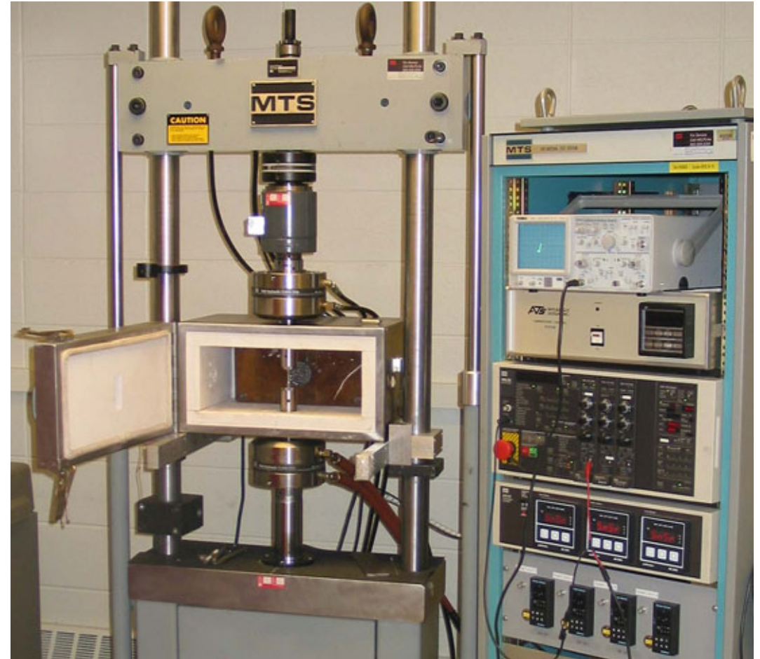
Fig. 5.6 Closed-loop servo-controlled hydraulic testing system
